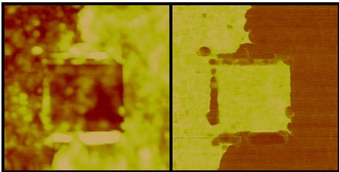
suggests that some ill-defined surface mixture of the two components has not resulted: the level of friction within the cleared region is equal to the level of friction found in the initial exposed underlayer region at left. (Intermediate values are indeed found within the lip of material piled at the periphery of the cleared region.)
